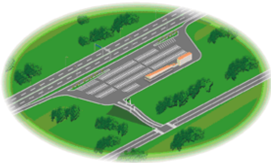
Figure 4.3-6 Example of smart IC (Miyoshi smart IC in Kanetsu Expressway) (Source: MLIT)
