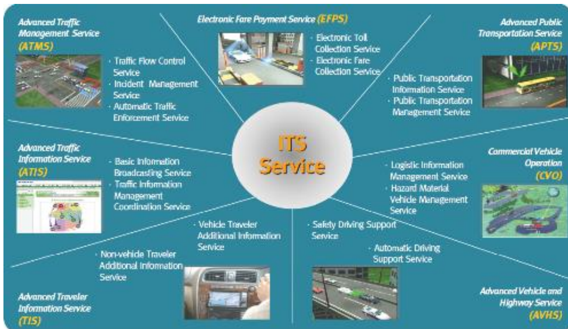
Figure 5.1-2 ITS Architecture and Services
