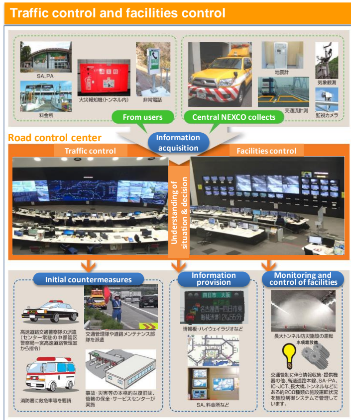
Figure 4.1-3 An example of traffic control center (Source: Central Nippon Expressway Company Limited)
